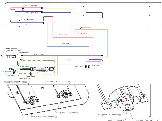
NOTE: THE LED DRIVER IN THIS FIXTURE IS DESIGNED TO OPERATE ON GROUNDED NEUTRAL SYSTEMS ONLY. IMPORTANT SAFETY NOTE: THERE IS STILL VOLTAGE INSIDE THE FIXTURE WHEN THE FIXTURE IS OPENED. WARNING: TO PREVENT THE RISK OF ELECTRICAL SHOCK DEACTIVATE/DISCONNECT THE POWER SUPPLY BEFORE MAINTENANCE OF FIXTURE.
