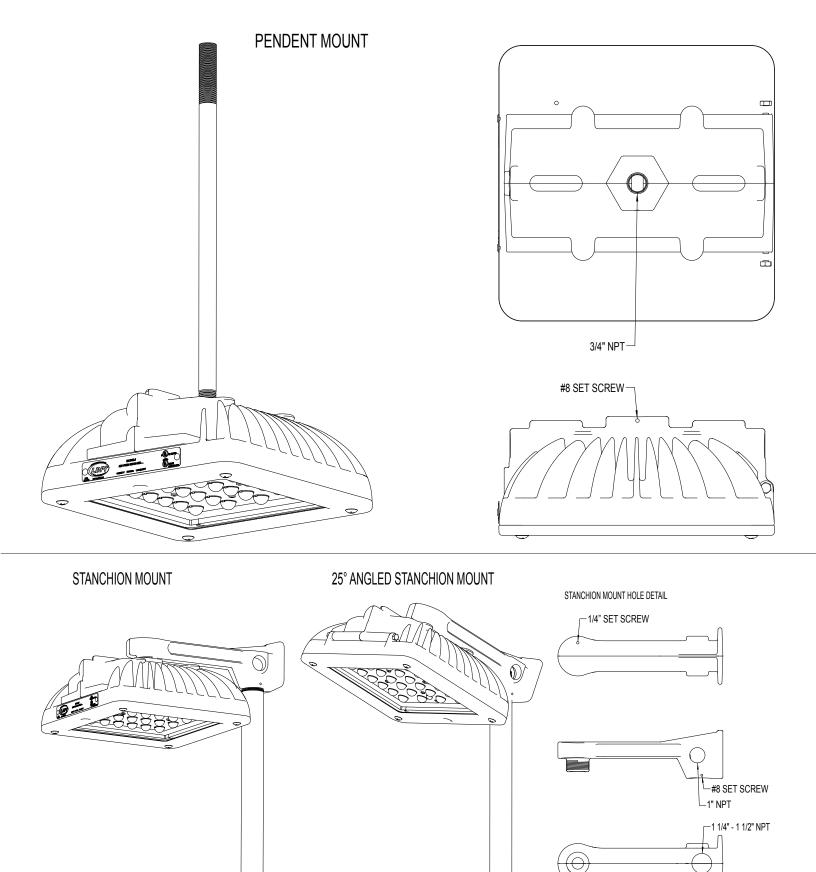
Securely tighten set screws when desired luminaire orientation is achieved and the conduit connection is tight.
